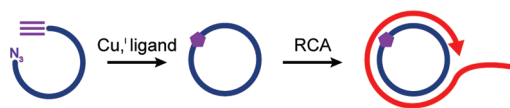
FIGURE 2. Click DNA cyclization and rolling circle amplification (RCA) through triazole linkage B.
